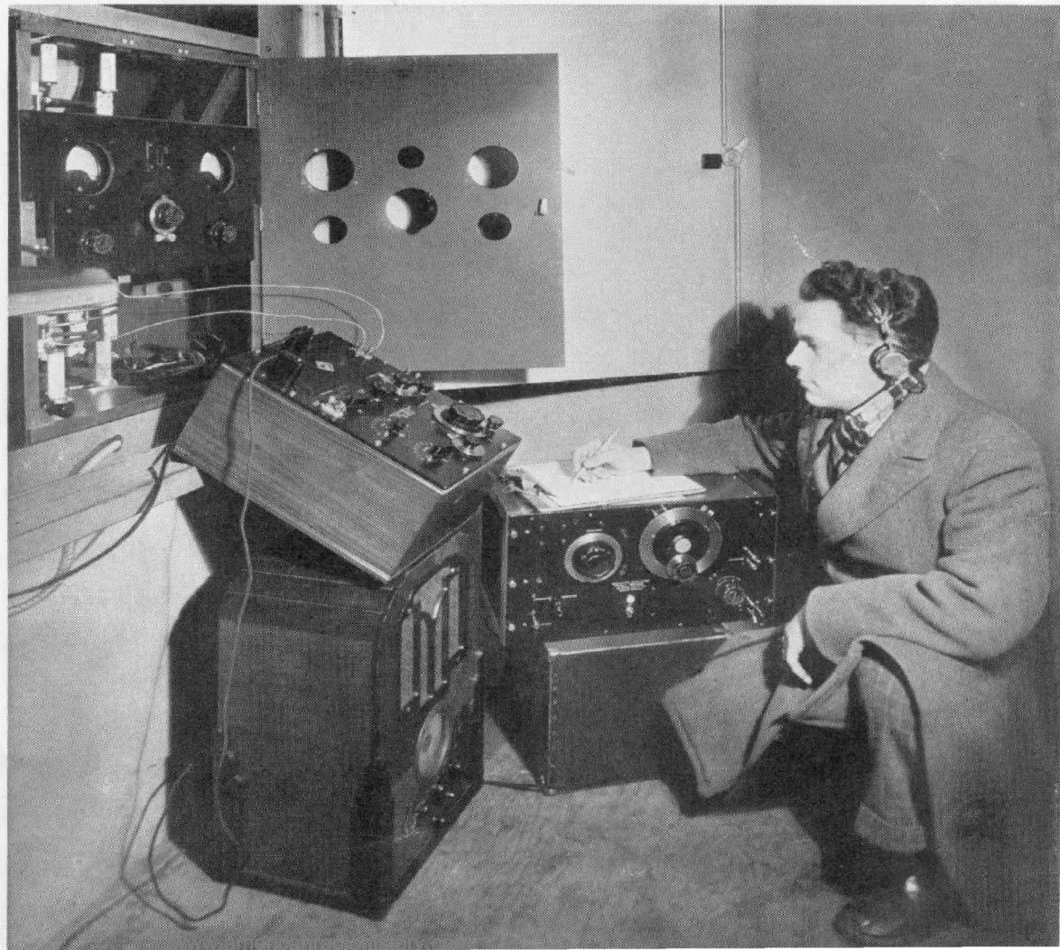
FIGURE 6. This photograph shows the radio-frequency bridge, the modulated oscillator, and radio receiver set up in the "dog house" at the base of the antenna. The equipment at the extreme left of the picture includes the impedance-matching networks and meters for reading antenna current
